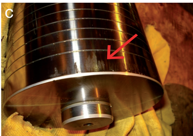
Fig. 9: Step-two piston with cavitation
