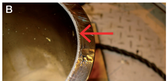
Fig. 8: Step-one piston with cavitation
