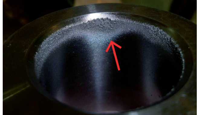
Fig. 7: Lower thrust piece with cavitation
